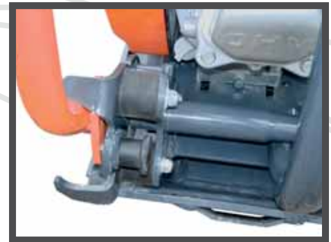
HANDLE LATCH FOR INCREASED STABILITY WHILST OPERATING THE WHEEL KIT
